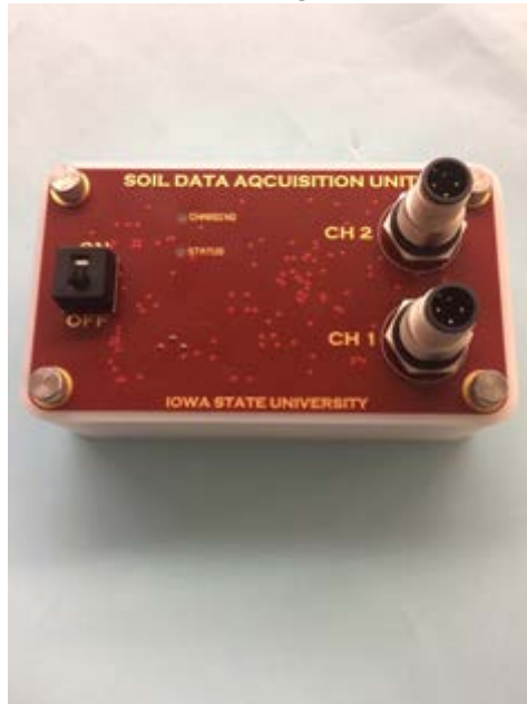
Figure 6: DAQ assembly with thumb screws installed
