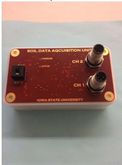
Figure 5: DAQ PCB placed on top of enclosure
