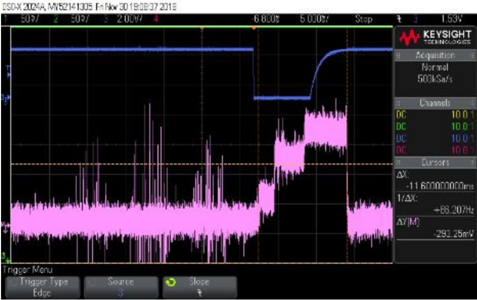
Figure 2: Oscilloscope screen shot for sleep and wakeup test. The blue waveform is monitoring the interrupt signal generator output of our real time clock IC. The pink waveform is a differential probe signal across a resistor which can then be used to measure a current draw and obtain power used by the system. Note that when the system wakes up (when the blue signal goes low) the current draw is not constant and is only for a short time period (~11.6 ms).
