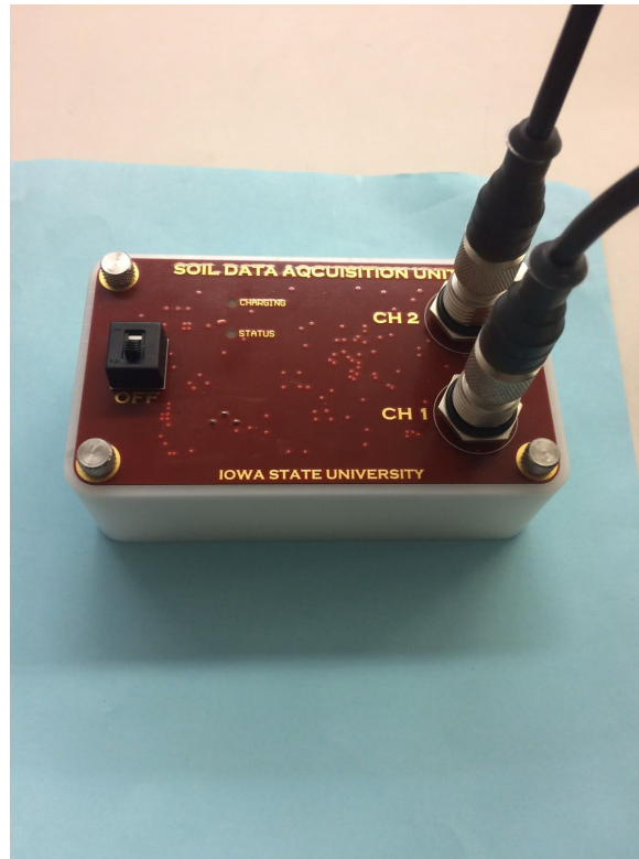
Figure 1: Fully assembled DAQ system mounted to custom enclosure.
